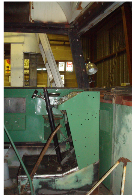
This photo shows the dash and adjacent wall panels mounted above the new driver’s platform flooring in September 2011
