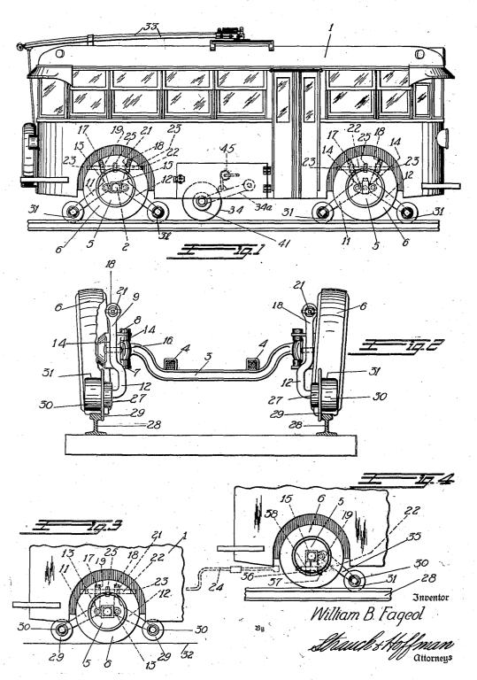
PNEUMATIC TIRE COMBINATION RAIL AND HIGHWAY UNIT
